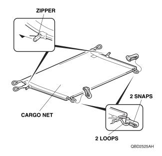
Attach four loops from the cargo net to the two anchors.
